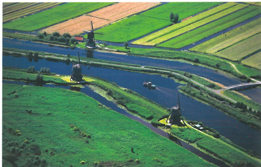
▲ FIGURE 1-44 SUSTAINABLE ECOSYSTEM: THE NETHERLANDS (left) The Dutch people have considerably altered the site of the Netherlands through creation of polders and dikes. (right) A polder in North Holland has been created by pumping the water from the site into the canal.
